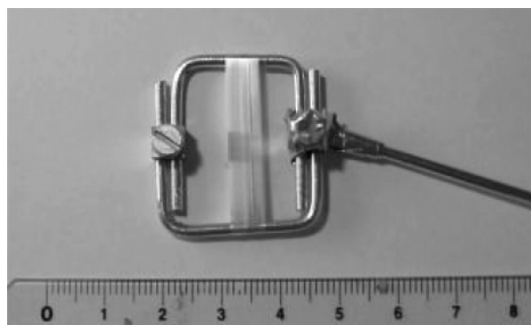
Figure 1. Photograph of spider dragline silk (mass about 20 mg) wound on an aluminum frame sample holder.
